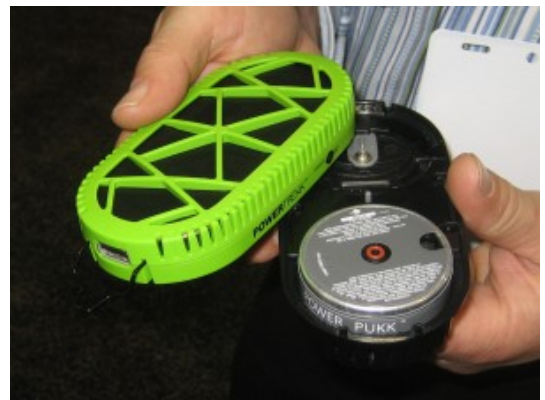
The PowerTrek lid can also be charged via USB without the fuel-cell system.
