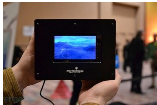
MasterImage's parallax barrier is also switchable, allowing the device to be rotated between landscape and portrait modes.
